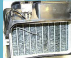
Thermostatic switch installed in evaporator coil
